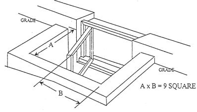
The clear horizontal dimensions shall allow the window to be fully opened and provide a minimum accessible net clear opening of 9 square feet, with a minimum dimension of 36".
